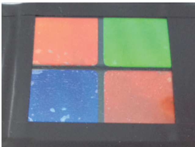
Figure 6. Color reflector with double layer structure by the pixel division method.
